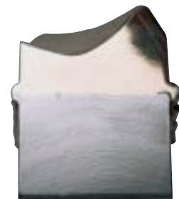
Section of electron beam welded wormwheel rim and centre showing the fusion of the bronze wormwheel rim onto the cast iron centre. This high security fit allows transmission of power under shock load conditions.
