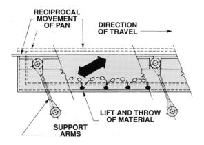
The pan arm provides the necessary linkage to support and isolate the trough between the base structure.
